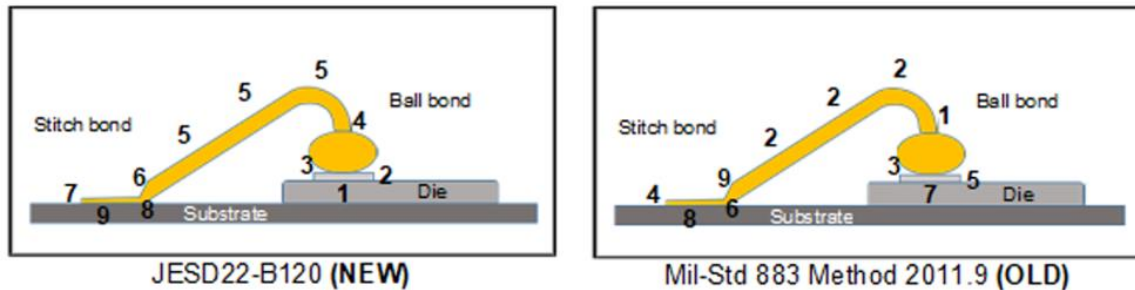
Figure 32 – Pull Failure Code Locations for JESD22-B120 and Mil-Std 883 Method 2011.9
