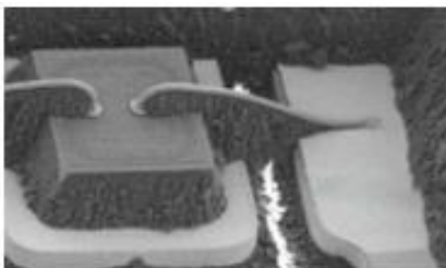
Figure 25 – Laser Ablation Damage
