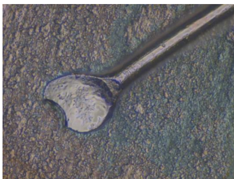
Figure 28 – Ag Plating Removed by the Decapsulation Process, Underlying Cu is Visible
