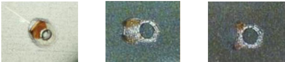
Figure 35 – Examples of Break Occurring Within the Neckdown Region
